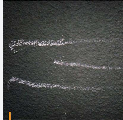
ASTM D3363 - Scratch/Gouge
